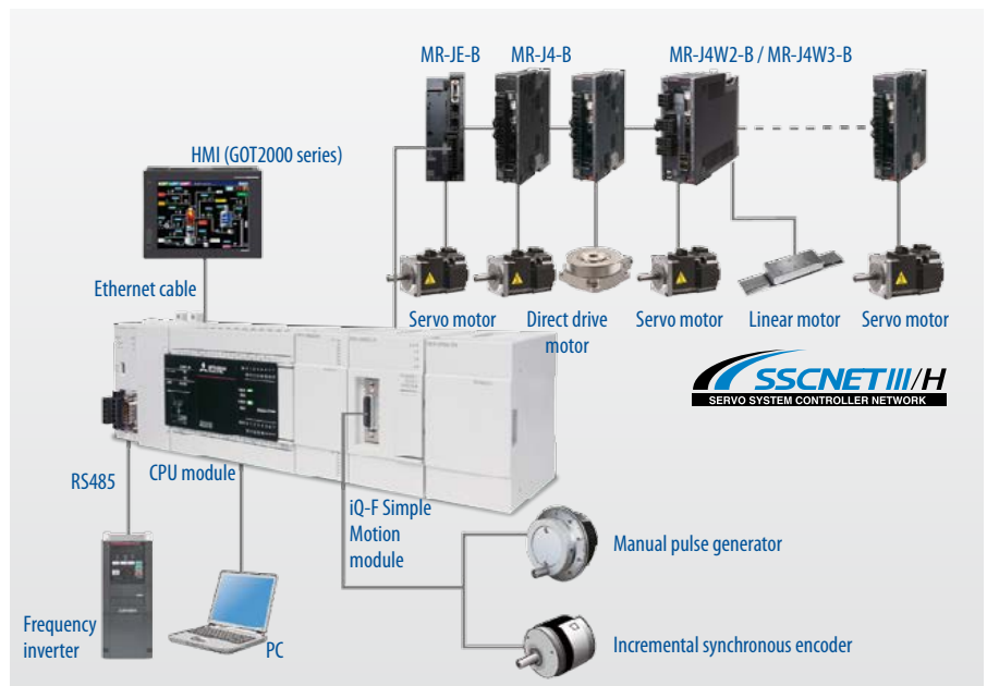
Structure of a system configuration comprising servo amplifiers and servo motors together with an MELSEC iQ-F PLC-CPU.
